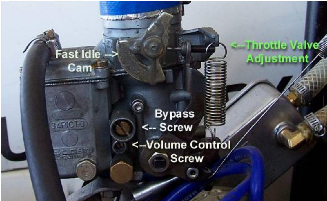
On the First carb you have lots more adjustment screws than on the old FV carb. There is a *throttle valve adjustment* screw at the end of the long arm attached to the throttle pivot. There is a large adjustment screw called the *bypass screw* and a smaller screw called the *volume control screw*.
